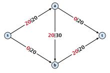
From the graph G = (V, E, c) and the current flow f we construct an auxiliary graph  $G_f = (V, E_f, c_f)$  (the residual graph):
