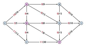
A node that has  $\sum_{e \in \text{out}(v)} f(e) < \sum_{e \in \text{into}(v)} f(e)$  is called an active node.
