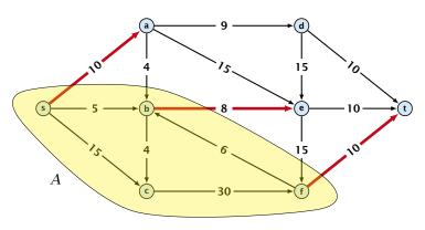
The capacity of the cut is  $cap(A, V \setminus A) = 28$ .
